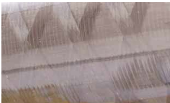
Figure No.2: Axial layer visible between the crossings of a partial helical layer.
